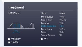
Ramp powered mode with adjustable rampup, ramp-down and plateau time.
